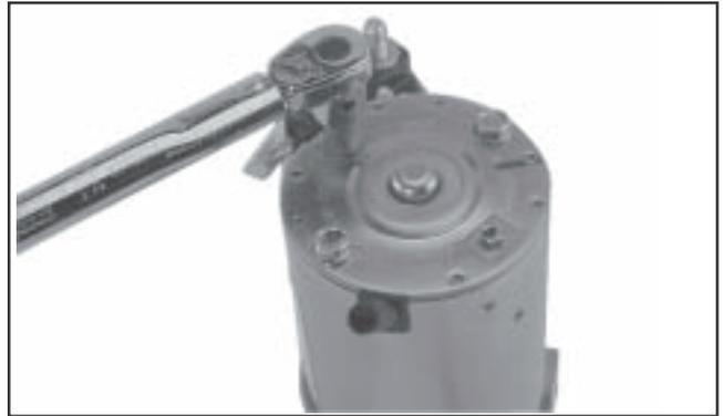
Figure 8-56. Torquing Brush Holder Screws.
