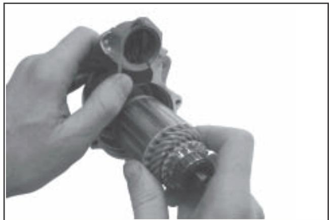
**Figure 8-21. Installing Armature.**
