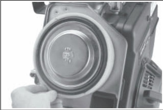
Figure 11-59. Installing Air Cleaner.
