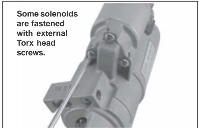
Figure 8-30. Removing Solenoid Screws.
