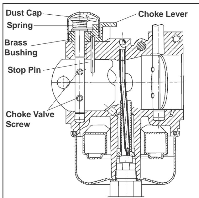
**Figure 5-15. Cutaway View Showing Self-Relieving Choke Carburetor.**
