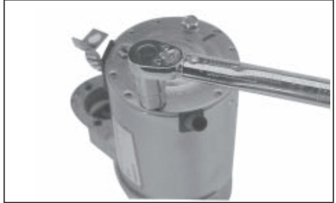
Figure 8-55. Torquing Thru Bolts.
