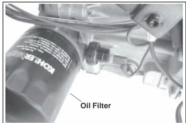
Figure 6-4. Oil Filter and Oil Sentry™.
