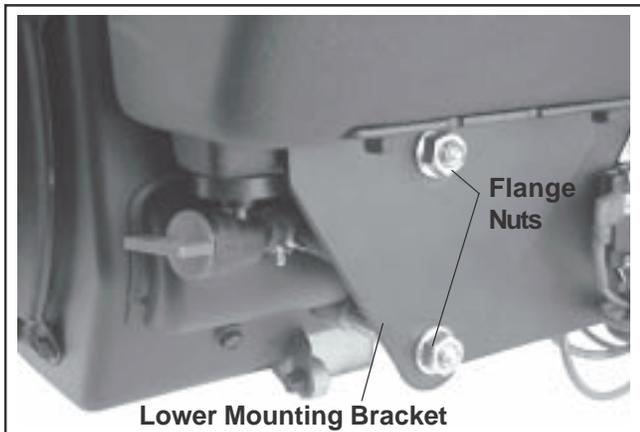
Figure 11-51. Installing Fuel Tank Lower Mounting Flange Nuts.
