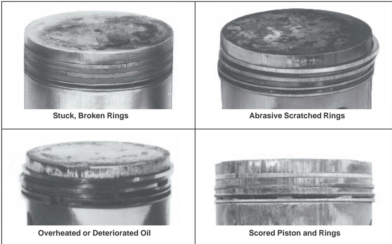
**Figure 10-5. Common Types of Piston and Ring Damage.**
