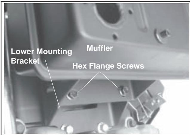
Figure 9-3. Removing Muffler.
