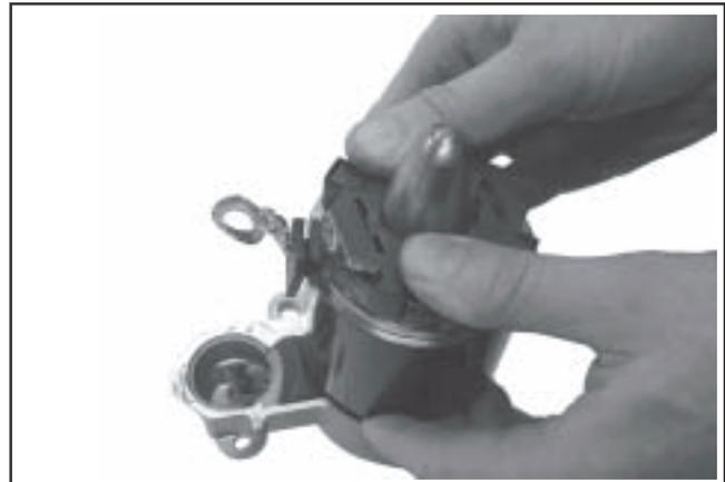
**Figure 8-25. Installing Frame with Brush Plate Assembly.**
