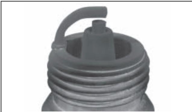
**Carbon Fouled:** Soft, sooty, black deposits indicate incomplete combustion. Incomplete combustion is usually caused by overrich carburetion, weak ignition, or poor compression.
