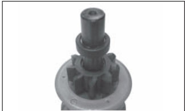
**Figure 8-20. Lock Collar around Retaining Ring.**
