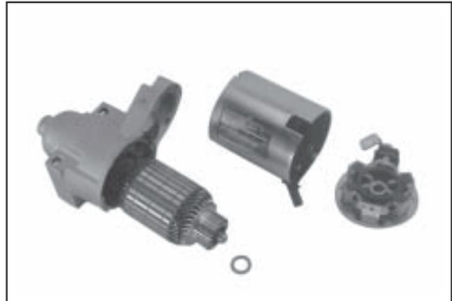
**Figure 8-35. Starter Frame Removed.**
