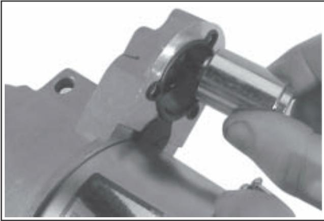
**Figure 8-32. Removing Plunger.**
