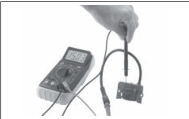
**Figure 8-4. Testing Module Secondary.**
