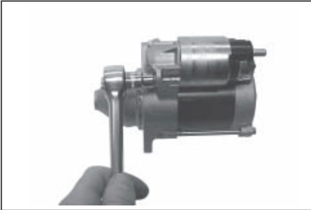
Figure 8-27. Installing Solenoid.
