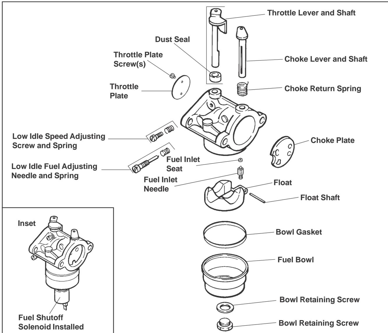
Figure 5-8. Adjustable Main Jet Carburetor - Exploded View.
