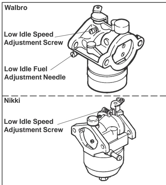
Figure 5-4. Carburetor Adjustment.
