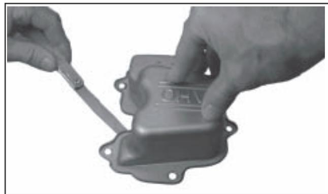
Figure 10-11. Checking with Feeler Gauge.
