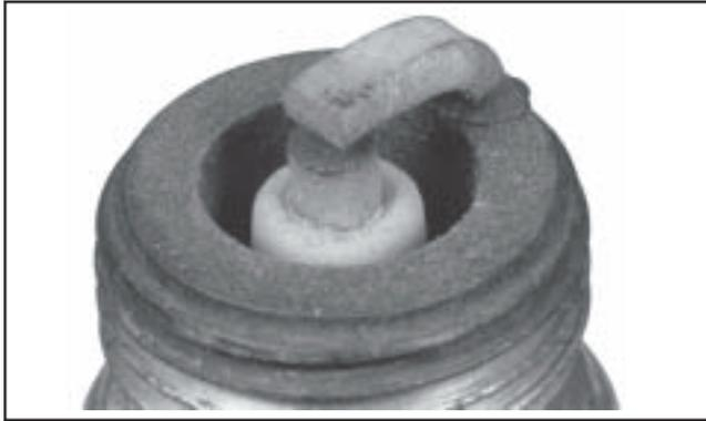
**Normal:** A plug taken from an engine operating under normal conditions will have light tan or gray colored deposits. If the center electrode is not worn, a plug in this condition could be regapped and reused.
