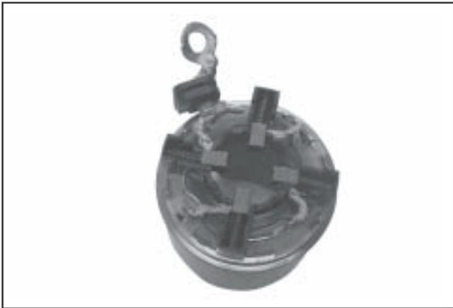
**Figure 8-22. Mounting Brush Holder to Frame.**
