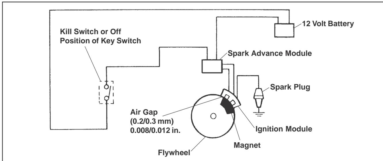
Figure 8-5. Capacitive Discharge Ignition System with Spark Advance.
