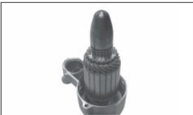
**Figure 8-24. Tool on end of Armature.**
