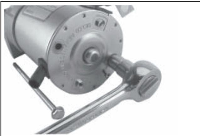
**Figure 8-33. Removing Thru Bolts.**
