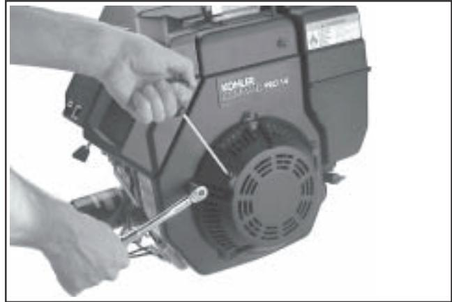
Figure 11-61. Installing Retractable Starter.
