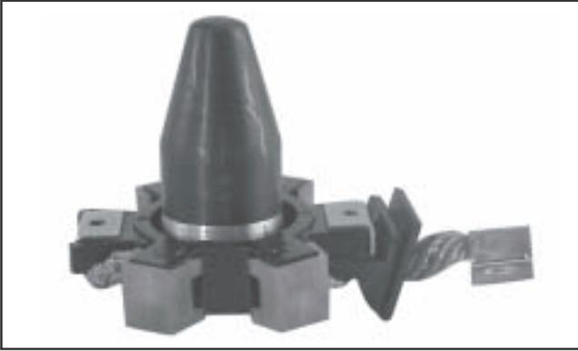
Figure 8-53. Brush Installation Tool with Extension.
