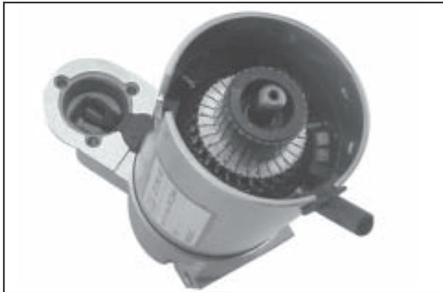
**Figure 8-49. Installing Frame and Drain Tube.**
