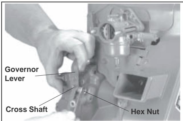
**Figure 5-18. Governor Adjustment (Air Cleaner Removed for Clarity).**
