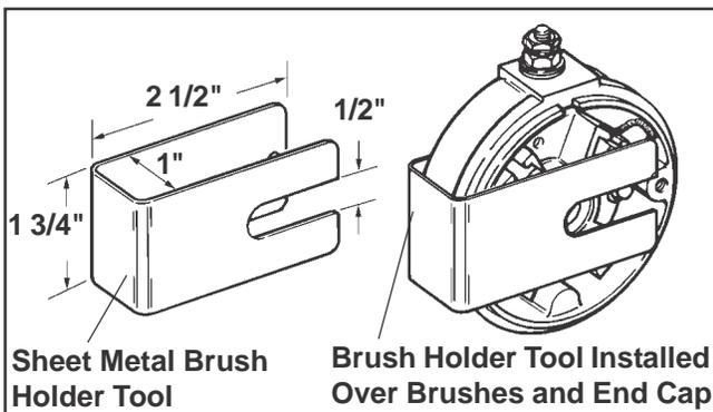
Figure 8-16. Brush Holder Tool (Style "A" End Cap).
