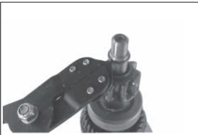
**Figure 8-39. Removing Retaining Ring.**
