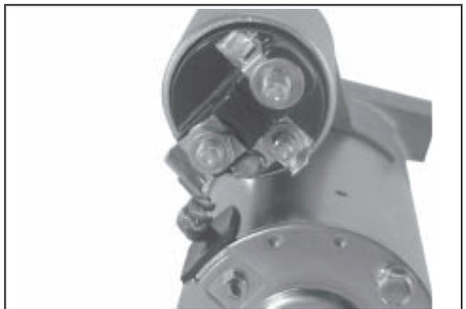
Figure 8-57. Positive (+) Brush Lead Connection.
