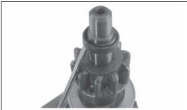
**Figure 8-45. Installing Stop Collar/Retainer.**
