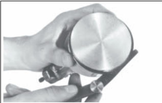
Figure 10-7. Measuring Piston Ring Side Clearance.
