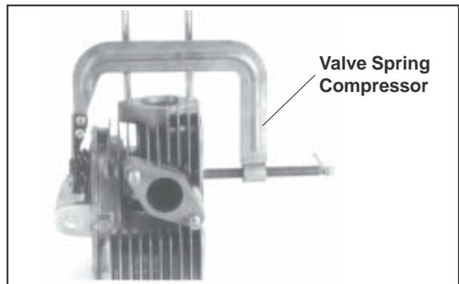
**Figure 9-34. Removing Valves With Valve Spring Compressor.**
