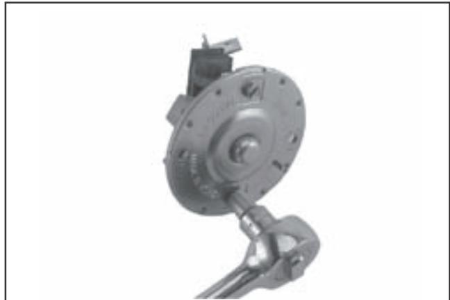
Figure 8-43. Removing Brush Holder.
