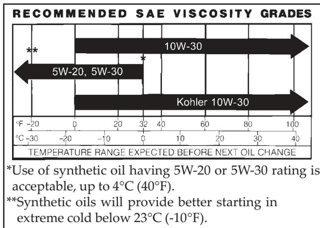
**NOTE:** Using other than service class SG, SH, SJ, or higher oil or extending oil change intervals longer than recommended can cause engine damage.
